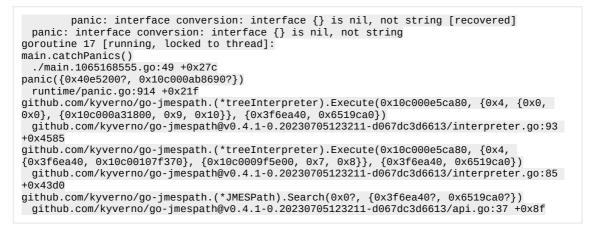
This part of Kyverno is invoked as part of the image verification by *imageverifier.verify*. Below, HasChanged() invokes the faulty execution path:
